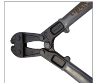
Ø 12 mm max cutting capacity
